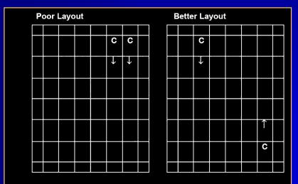
**Figure 3.** Potential plate layouts in a typical multiwell-plate assay. C indicates calibrator, with dilution increasing in the direction indicated by the arrow.
